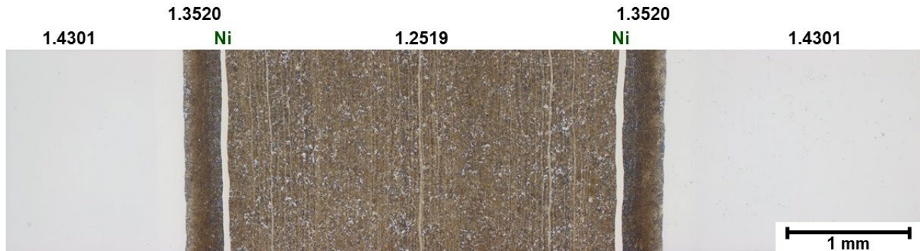
Fig. 1 Composite after forging the starting sheets and before forging to final knife blade dimension. Overview images of the cross-section etched with Nital.
