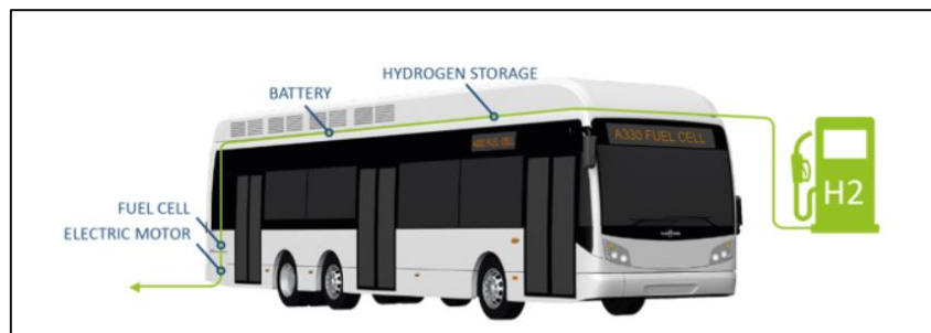
Figure 5: How an hydrogen fuel-cell bus works (Source: https://www.fuelcellbuses.eu (2020)) 7
