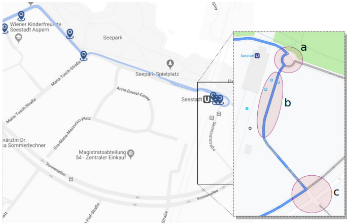
Figure 4.9: Evaluation areas in Seestadt Aspern. The zoomed-out map shows the official driving route of the bus. The displayed detail of the map figures essential evaluation areas. Each area is focused on a specific scenario: a) roundabout with 14 traffic signs, b) bus station with number of dynamic obstacles and c) traffic lights with different states.
