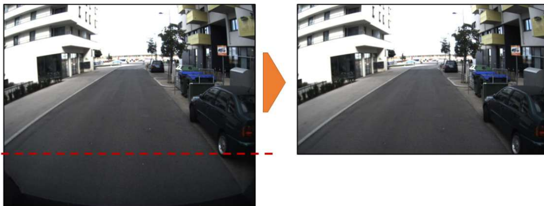
Figure 4.13: Example of an image recorded by the bus. On the left side the raw image is shown with the planned image cut and on the right side the cropped image is visualized.
