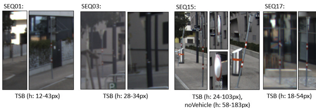
Figure 5.6: Traffic signs which are not detected by the object detection model. Five traffic signs within four subsequences listed with the traffic sign class and its height over the whole subsequence.
