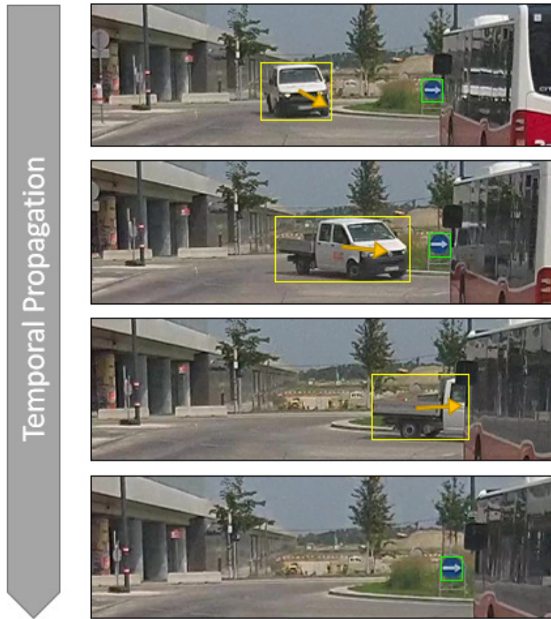
Figure 3.10: Example of occlusion handling: A detected moving object occludes a static object. Both object instances are detected correct.
