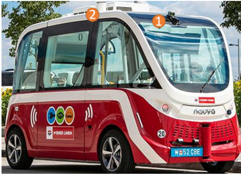
Figure 3.2: Autonomous bus from manufacturer Navya. A RGB camera is mounted on the upper side of the windshield (1). A GPS antenna is placed on top of the bus (2).
