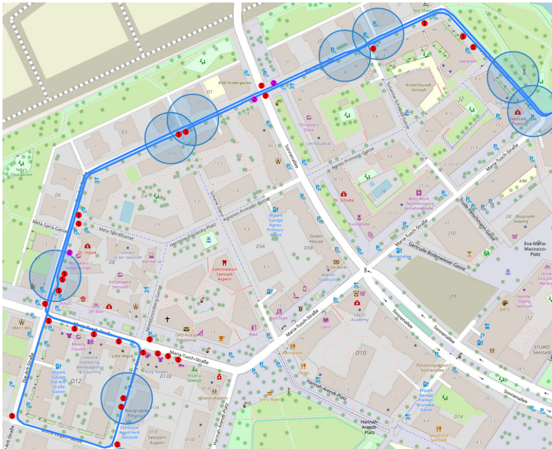
Figure 4.14: Seestadt Aspern GPS evaluation area. The blue circles indicate areas of bus stops whereby the red and purple dots are traffic sign locations. The red point indicates one and the pink two traffic signs on the same position.
