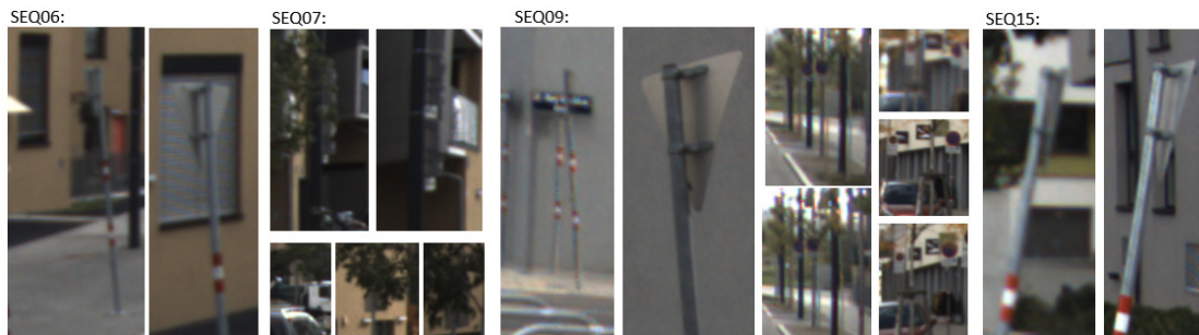
Figure 5.9: Missed localization signs due to missing predictions when performing object detection. The signs are mainly triangular-shaped signs from the back.
