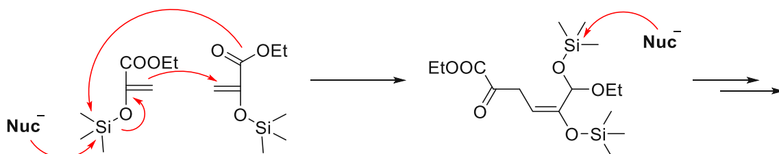
Figure 47: Group transfer polymerization of TMSA.
