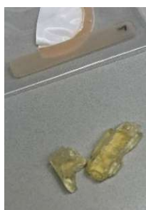
Figure 144: DMTA specimen before (above) and after (below) oxidation for the sample containing 50 mol% VDB with respect to TAI and the thiol TMT in an equimolar ratio of double bonds to thiol groups.
