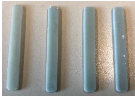
Figure 141: from left to right: DMTA specimens of polymerized formulations filled with 10 vol%, 20 vol%, 30 vol%, and 40 vol% of HAP.
