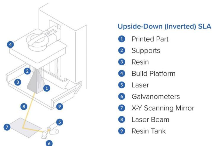
Figure 12: Principle of upside-down Laser-SLA. 94
