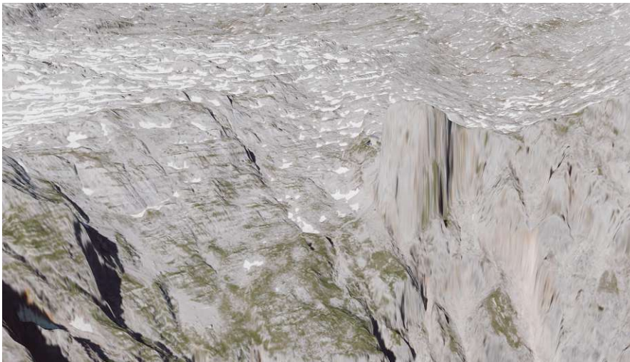
Figure 2.12: Orthoimagery draped on a 2.5D terrain. Note how in the near-vertical areas on the right, the texture is stretched.
