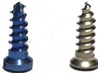
Figure 6: An example of the self-trapped screw (left) and a drill-free screw (right), each 2 mm in diameter and 6 mm in length [102].
