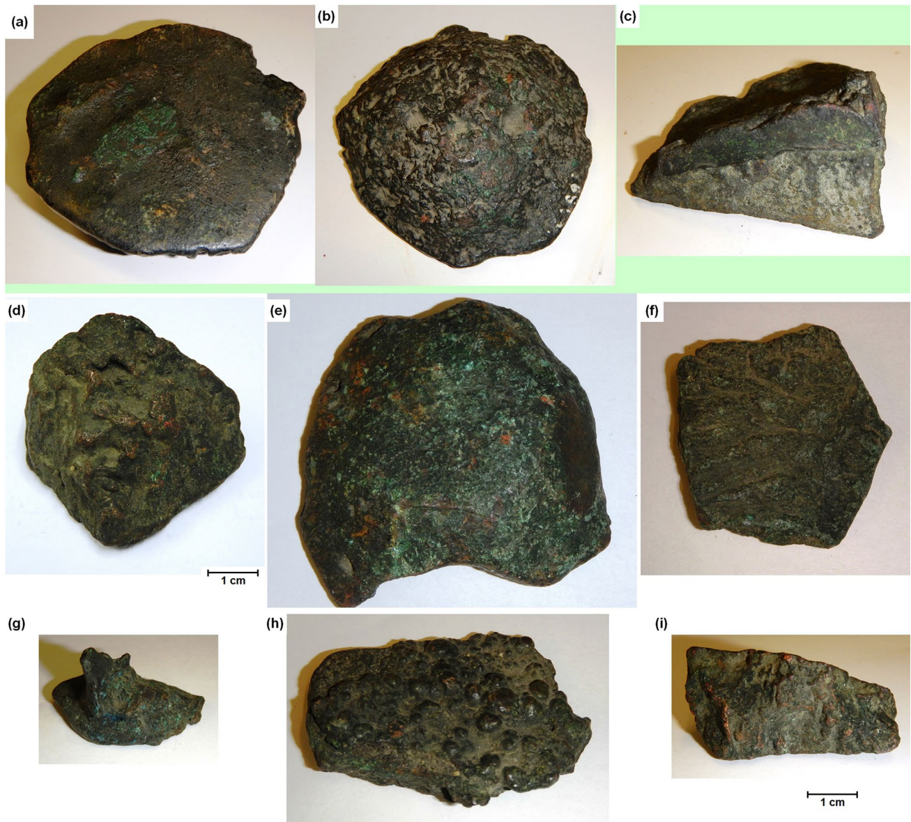
Fig. 1 Copper cast cakes (cc) from Drassburg. Whole cast cake a top, b bottom, c cast cake with a smooth surface from splitting, ( a–c ) not examined. Examined cast cakes d cc1, e cc2, f cc3, g cc4, h cc5, i cc6.
