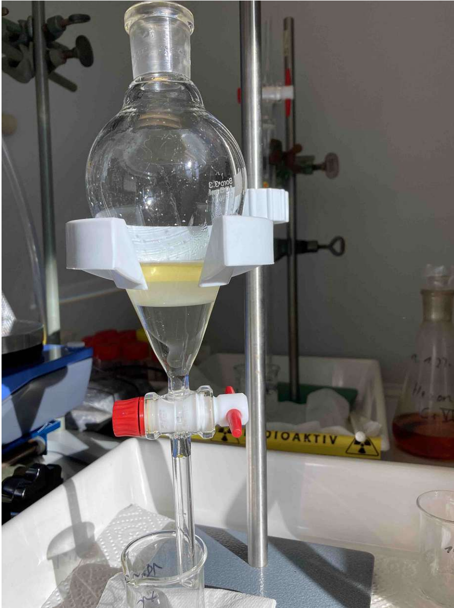
Figure 4.2: Liquid-liquid extraction of ammonium chromate in HCL in methyl isobutyl ketone: the lower aqueous phase is already almost colorless, the upper organic phase is yellowish. In between, a whitish emulsion can be seen in which the two phases are not separated from each other.
