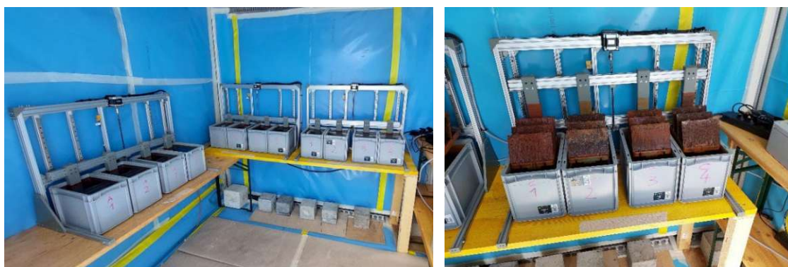
Figure 20: Alternate immersion in a temperature-controlled container [Paper III]
