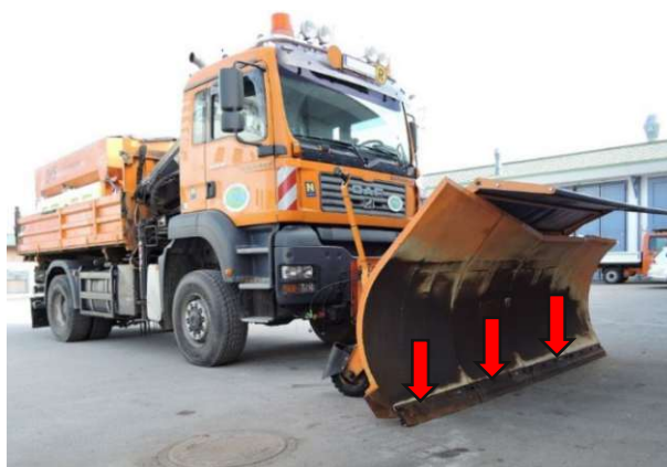
Figure 3: Removable snowplow blades (denoted by down arrows) on the snowplow
