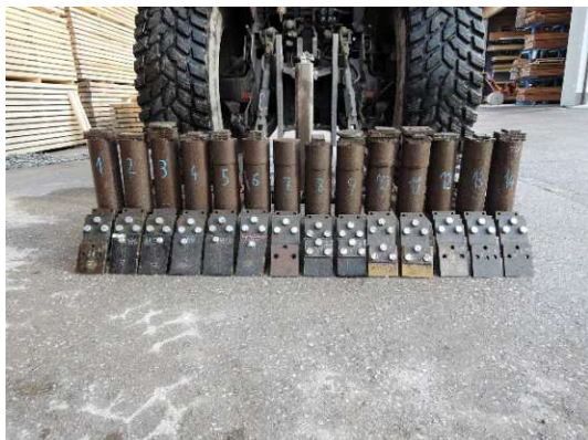
Figure 27: Test rack with snowplow blade segments [Paper IV]
