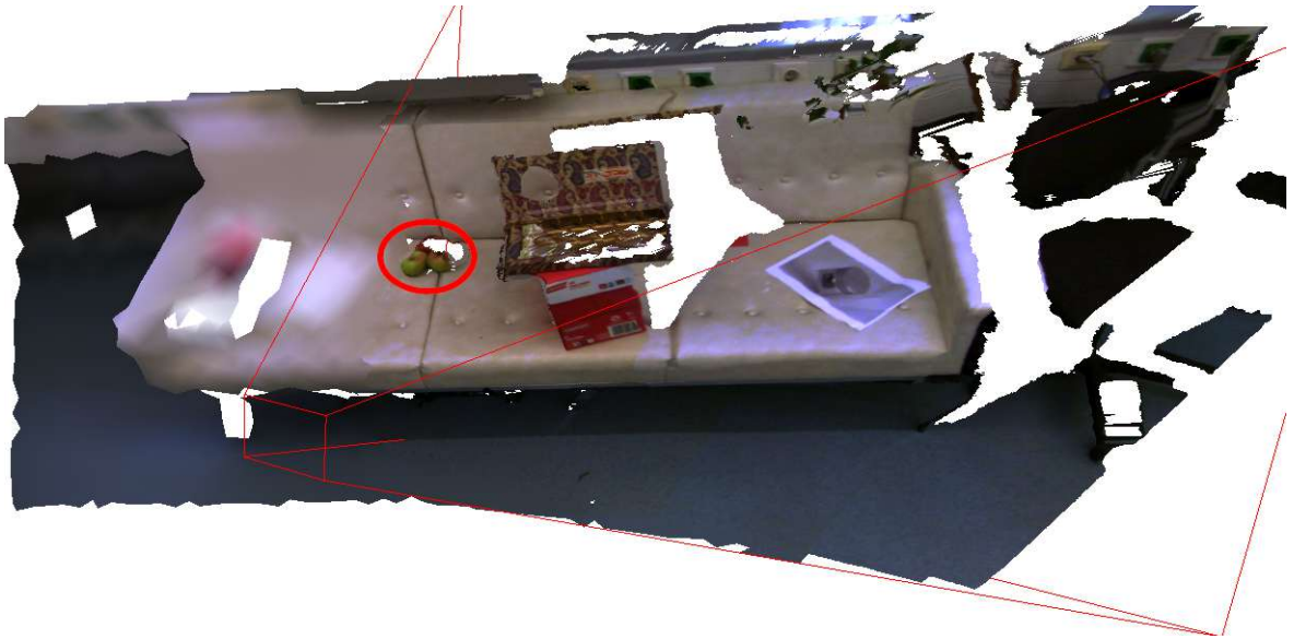
Figure 4.2: Demonstration of the Level of Detail system. The younger part of the reconstruction (right) resides in the memory of the GPU and is processed and displayed at full detail, while the older part (left) is downloaded to system memory and displayed with a low detail replacement. The apples shown in Figure 4.1 are taken from this reconstruction (red circle) and are meant to demonstrate the dynamic range of detail.
