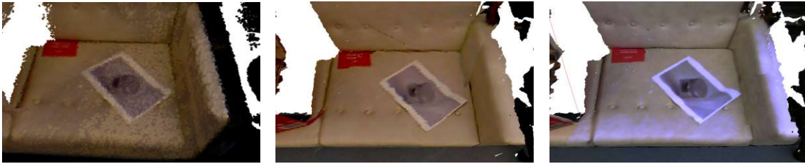
(a) ElasticFusion with Xtion-based RGB data. (b) ScalableFusion with Xtion-based RGB data. (c) ScalableFusion with high resolution RGB camera.
