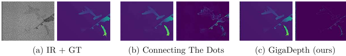
Figure 3.17: Disparities (left b, c) of the different algorithms on an artificial dataset based on models from [54]. Color-coding is applied for disparity errors (right b, c) of 0-5 pixel with outliers ( > 5 pixel) being black. (a) shows the input infrared image (IR) and ground-truth (GT).
