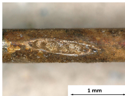
FIGURE 2 Mark of fretting observed at a wire from rope sample A1. [Color figure can be viewed at wileyonlinelibrary.com ]
