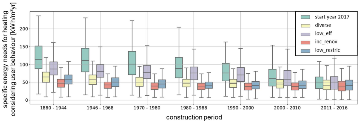
Fig. 10 Changes in specific energy needs considering user behaviour for heating in buildings from different construction periods between the base year and 2050 for all EU-27 buildings in the calculated scenarios
