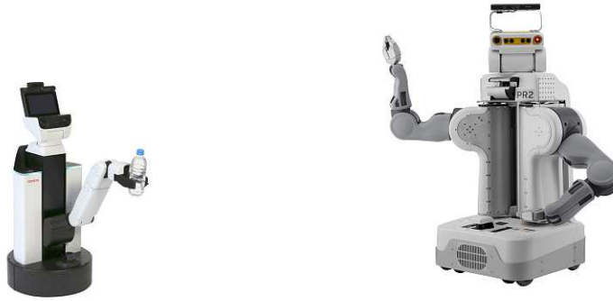
Figure 3.6: Two domestic service robots. Left: Toyota Human Support Robot (HSR). Right: PR2 by WillowGarage.
