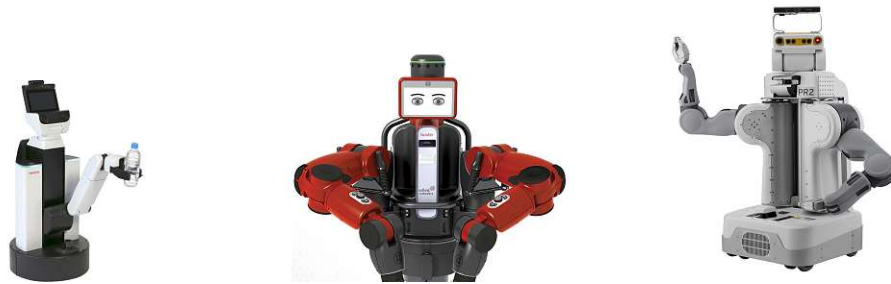
Figure 1.3: Three anthropomorphic service robots capable of object manipulation. Left: Toyota Human Support Robot (HSR). Middle: Baxter by rethink robotics. Right: PR2 by WillowGarage.
