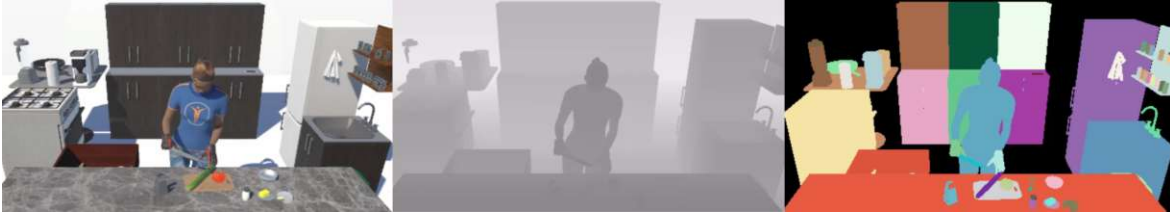
Figure 5.1: Dataset example for preparing salad. Left: RGB view; middle: depth view; right: object mask view.
