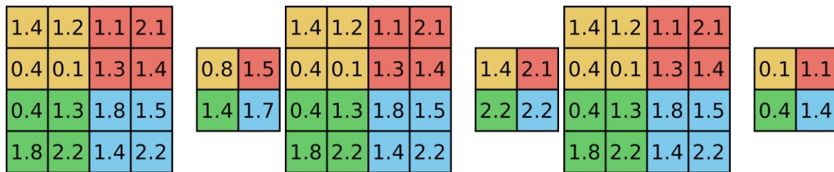
Figure 2.6: Pooling operations and how they operate. Adopted from [ 26, 4]. Shown is mean, maximum and minimum pooling.
