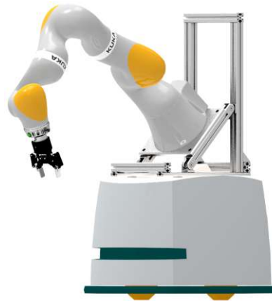
Figure 2.1: The modeled seven-axis mobile manipulator of the KUKA LBR iiwa R820 seven-axis manipulator mounted on the SALLY V2.0 mobile platform.
