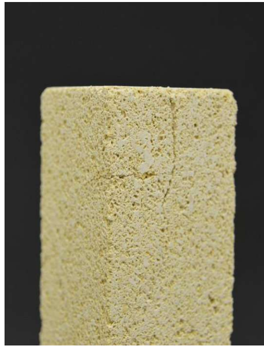
Figure S3. St. Margarethen after 14 cycles. Occurance of major cracks.
