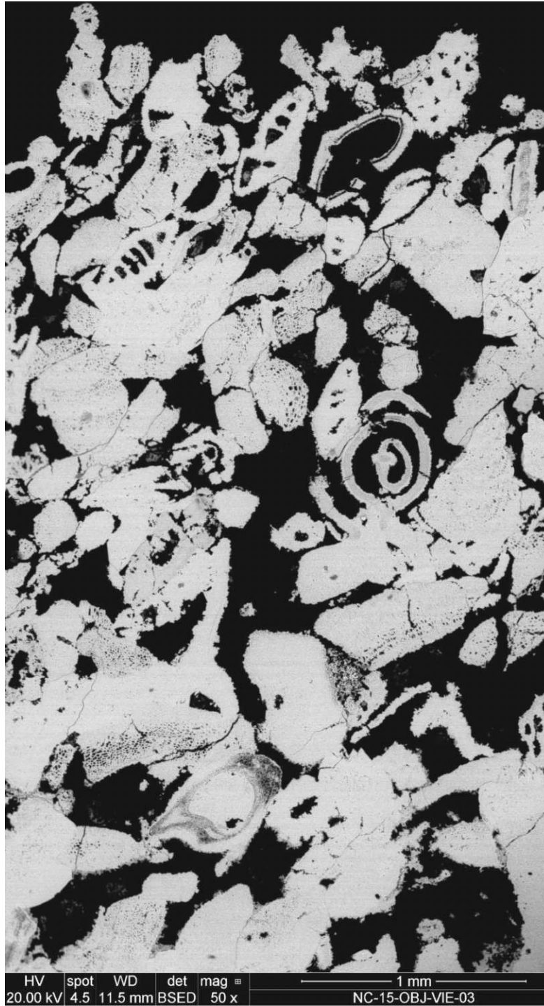
Figure S6. SEM-BSE, stitched micrograph, overview of dissolution effects (upper part of the sample), granular disintegration with inter- and intragranular micro cracks and the porous microstructure.
