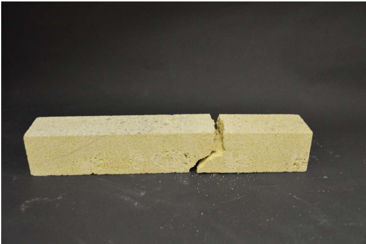
Figure S2. St. Margarethen after 56 cycles. Complete failure of the sample.
