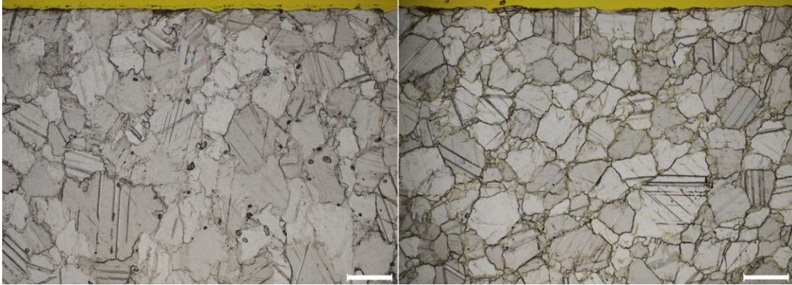
Figure S2c. Polarized microscope micrographs before ( left ) and after ( right ) thermal treatment of Apuan Marble. The fabric after thermal treatment displays mostly microcrack formation along grain boundaries. The scale bar is 200 \mu\text{m} .
