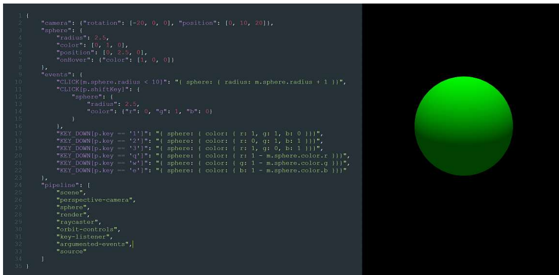
Figure 6.1: Case Study #1, Sphere. The left side shows the visualization description (enlarged in Listing 6.6), while the right side shows the resulting rendering. Changes to the description are immediately reflected in an updated visualization and vice versa.
