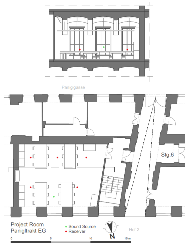
Figure 2.8: Section and plan of Panigtrakt. (●) Receiver positions during on-site measurements (●) Speaker position during on-site measurements
