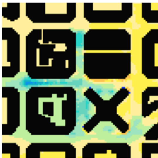
Figure 65. ENVI-met 2D temperature results for Sant Antoni at h = 1.5 m at 4:00
