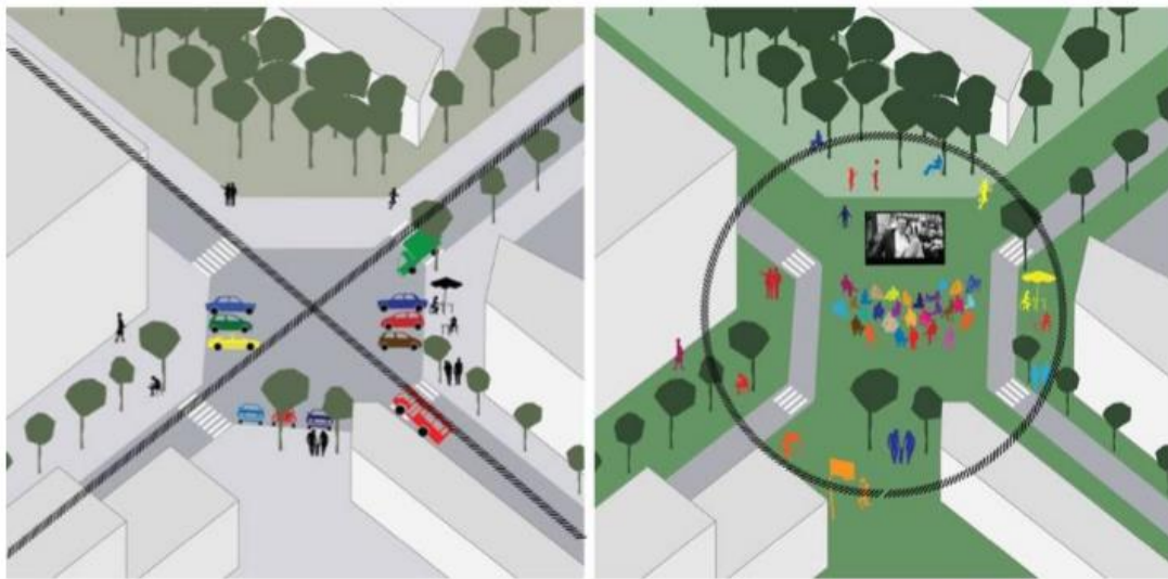
Figure 18. Schematic isometric view of an urban intersection, before and after the implementation of a Superblock (Rueda, 2016)
