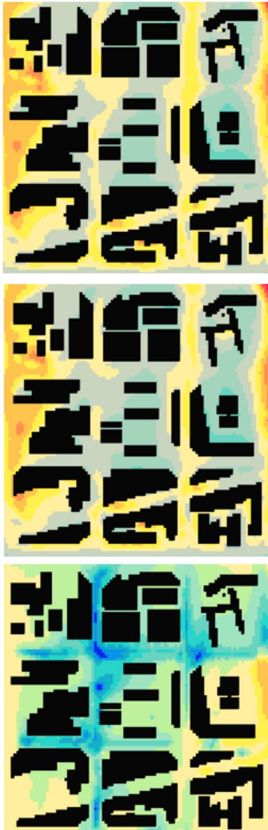
Figure 71. ENVI-met 2D temperature results for Poblenu at h = 1.5 m at 13:00
