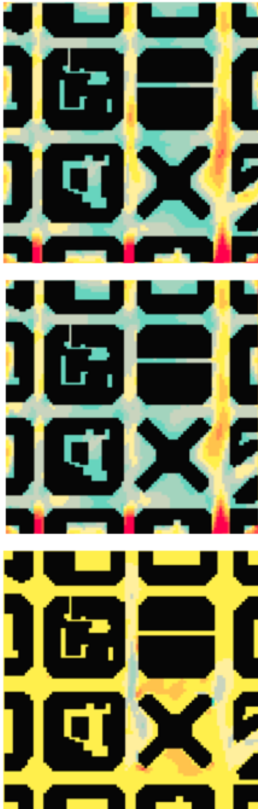
Figure 68. ENVI-met 2D air speed results for Sant Antoni at h = 1.5 m at 13:00
