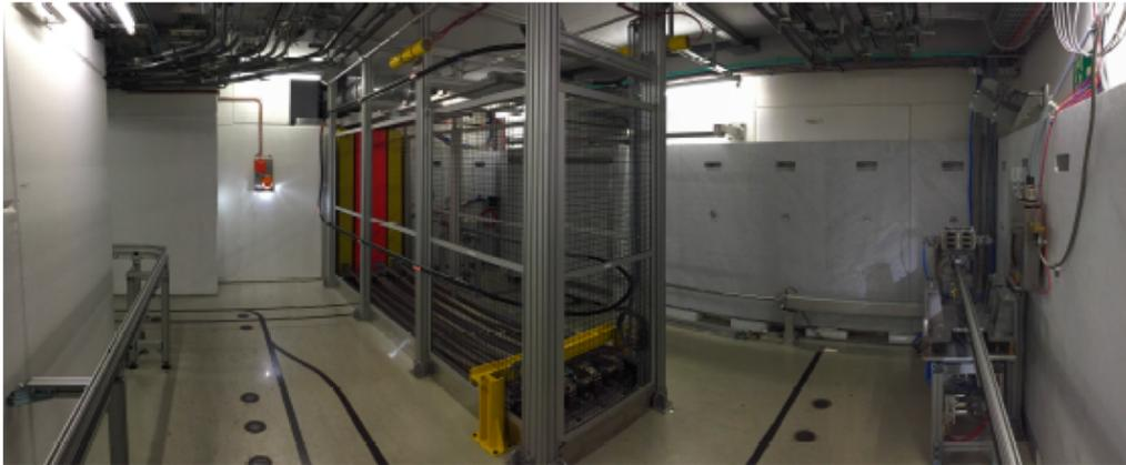
**Fig. A.1.:** Picture taken from inside the CHARM irradiation room. In the middle of the room, the shielding cage can be seen. The shielding layers are extracted in this pictures, but are still visible as yellow and orange slacks at the end of the cage. Additionally, the marble shielding, the rail for the Montrac test positions and the marked positions for the standard test positions, as dots on the floor, are visible.
