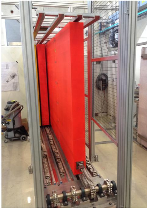
(a) Shielding cage and moveable shielding layers of CHARM. One iron layer is extracted right now.
