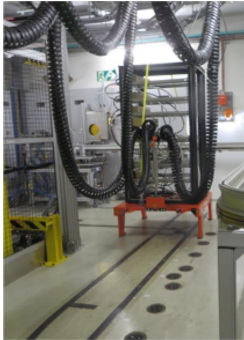
(b) Rack setup at one of the standard test positions. The cables to connect electronic devices are visible as well.
