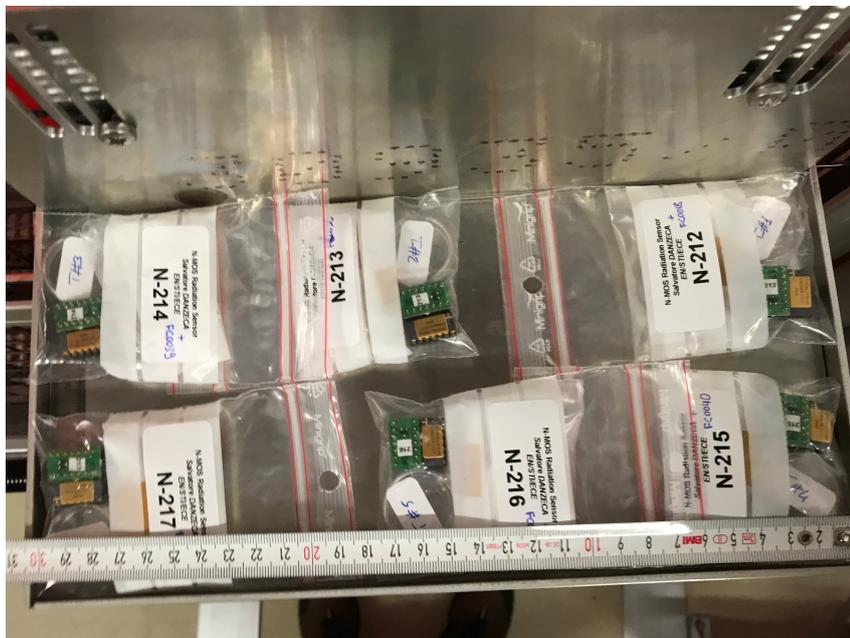
Fig. A.6.: Test setup for the test position T0. It can be seen that the dosimeter (RPL and RadFET) are covering the whole table.
