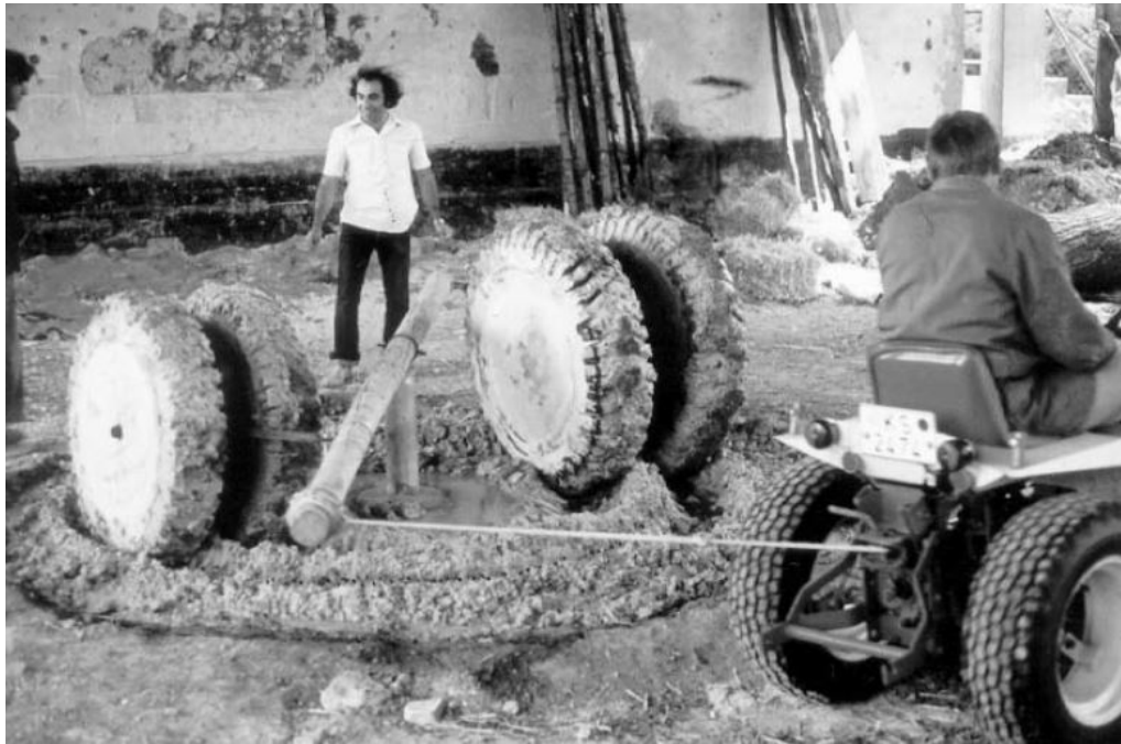
Fig.51: Mud wheel designed by the Building Research Laboratory (BRL) at the University of Kassel, Germany
