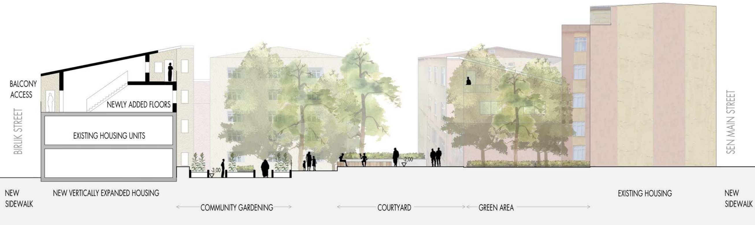
Fig 156 Relation between vertically expanded and existing housing and semi-public open space - Section 2-2
