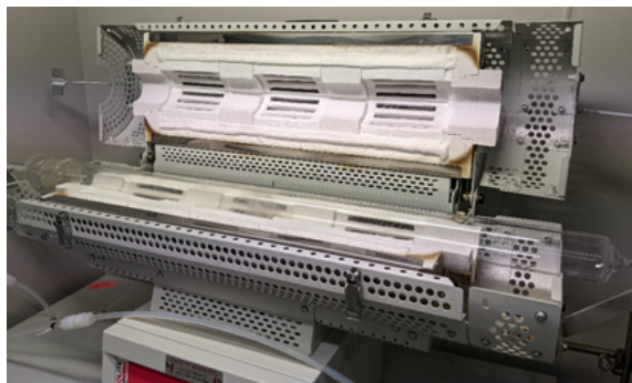
Figure 5.2: Carbolite EZS-3G floating furnace inside the fume hood.
