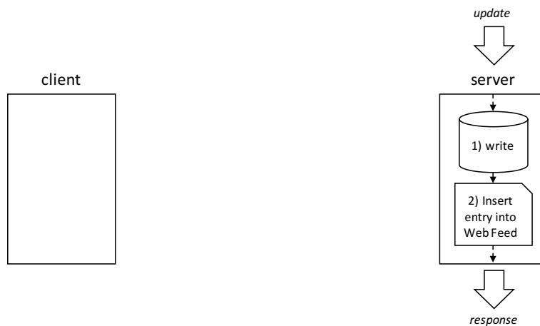
Figure 4.21: Procedure of an update with RS5
