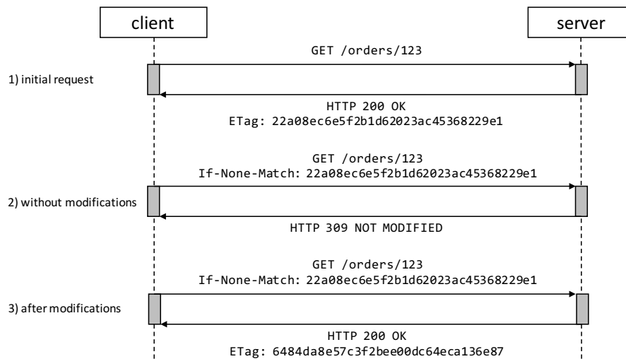
Figure 3.2: Example of the use of the ETag HTTP header
