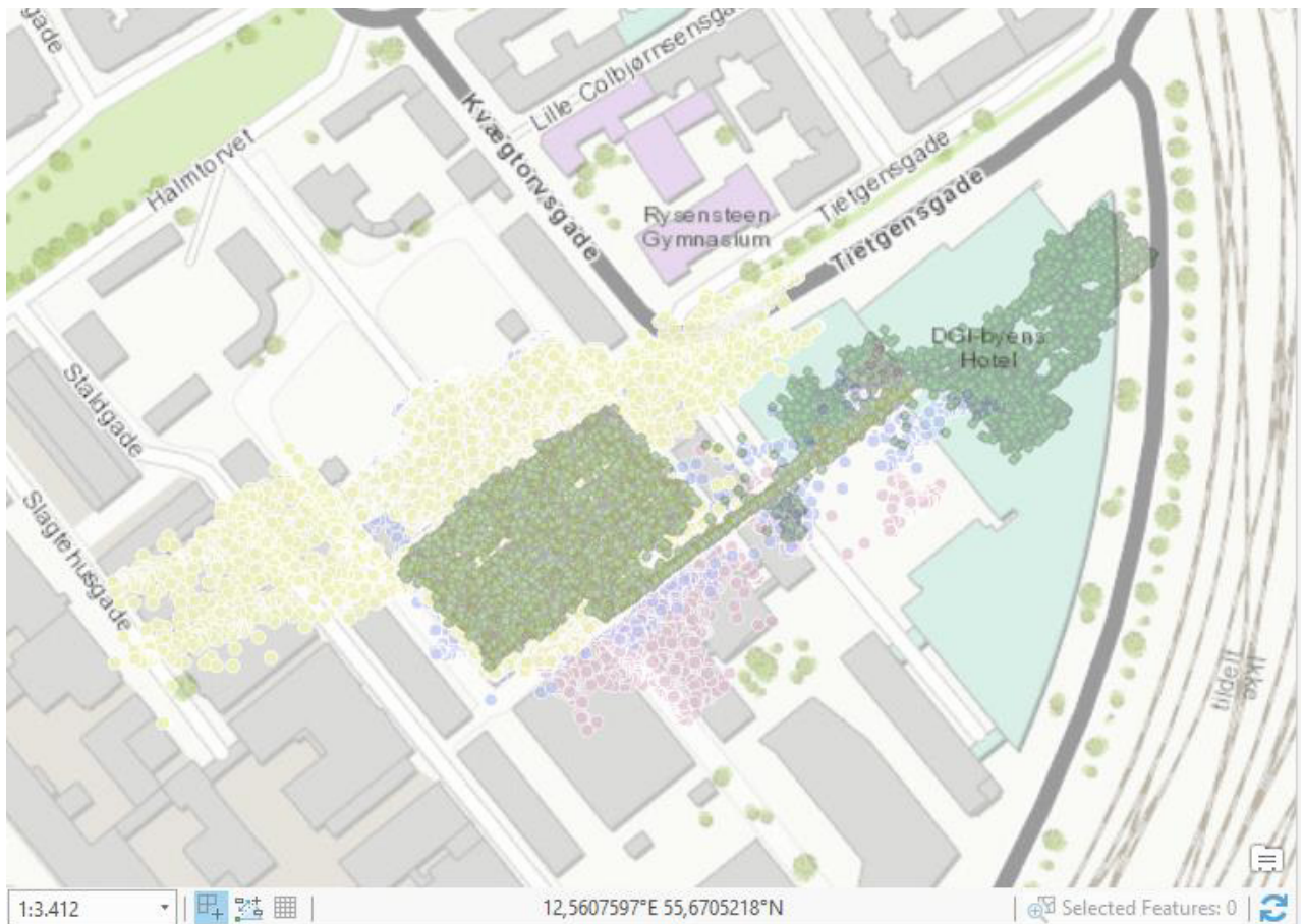
Fig. 15: Point Clouds after 7-Parameter-Helmert transformation
