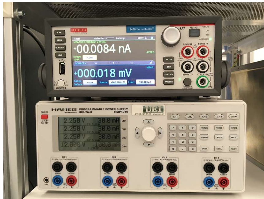
Figure 22: On top, the high voltage SMU ( Keithley 2470 ) can be seen that sits on the low voltage SMU ( Hameg HMP4040 )
