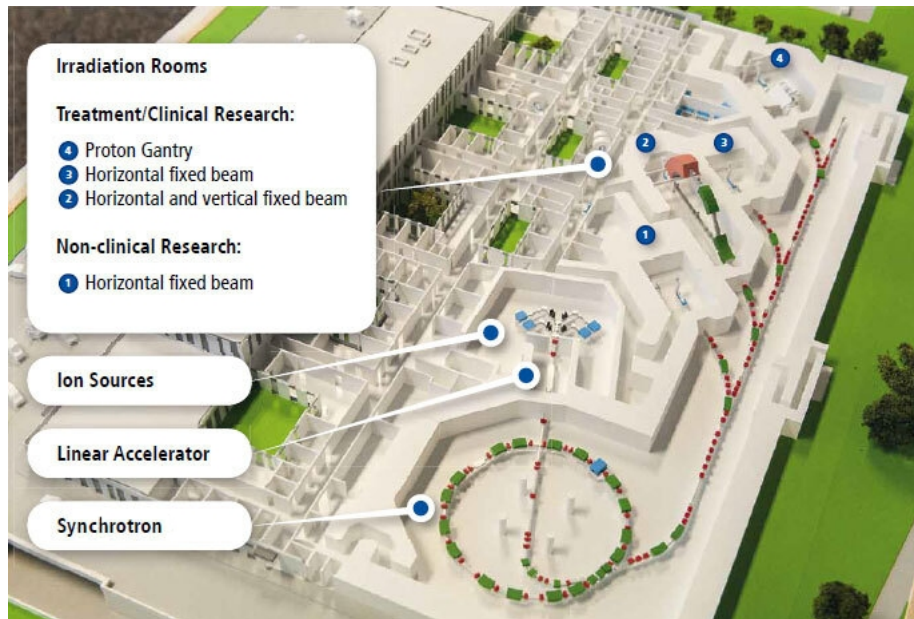
Figure 17: Layout of the MedAustron facility, where the ion sources, the linear accelerator and the synchrotron can be seen. Via magnets, the ion beam is guided to the irradiation rooms that are divided into clinical and non-clinical research [27].
