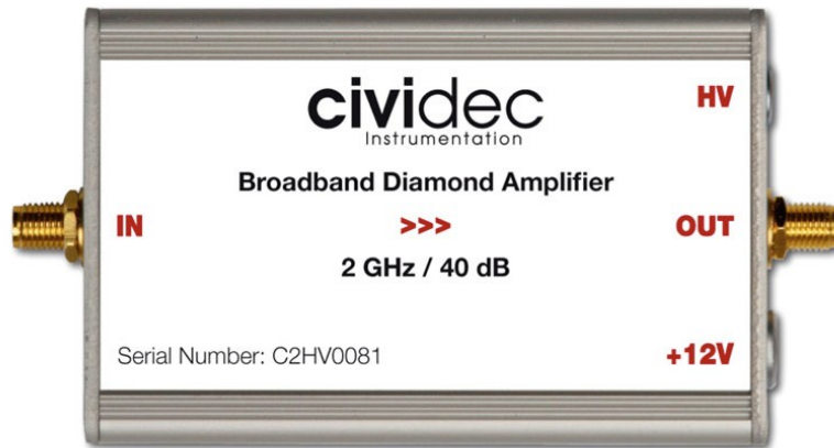
Figure 26: Front view of the cividec C2-HV Broadband amplifier that was used in the laser test for characterising it and in the first MedAustron experiment as a second stage amplifier [31].
