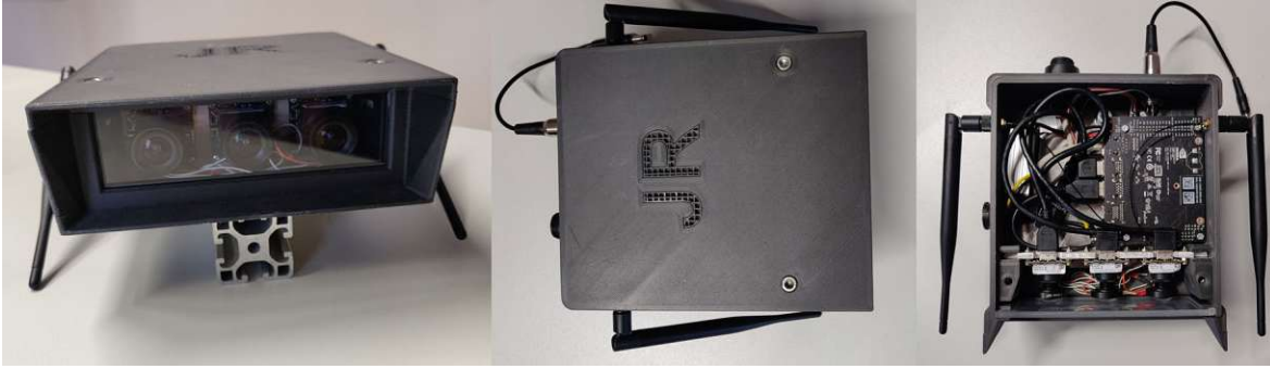
Figure 5.3: Cameras setup with two RGB cameras, a NIR camera and a NVIDIA Jetson Nano for inference of CNN models.
