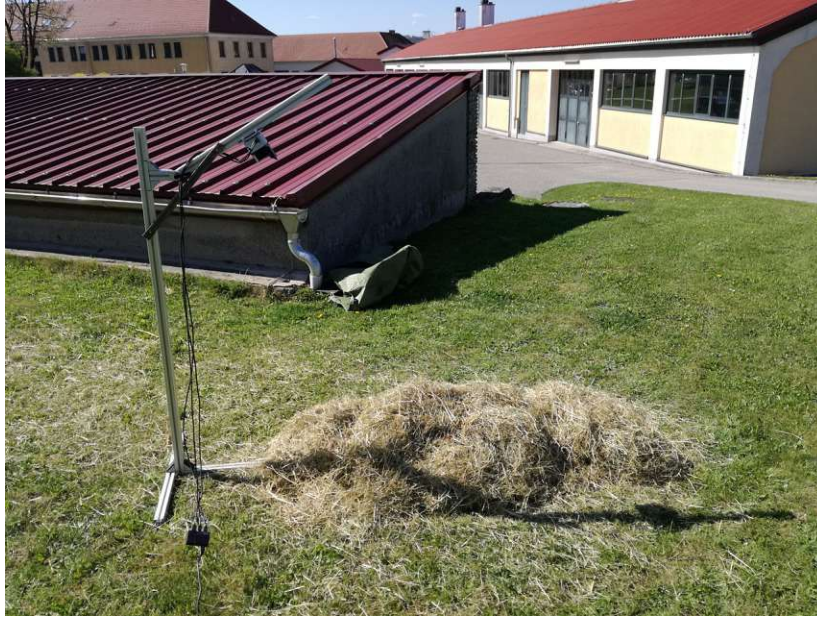
Figure 5.18: Outdoor laboratory trial to validate the swath measurement system under controlled conditions.
