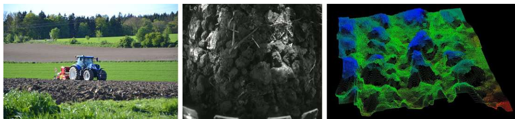
Figure 1.4: Left: Tractor with seed drill combination during seeding; Middle: camera view of the soil surface; Right: 3D stereo reconstruction of the soil surface for roughness estimation
