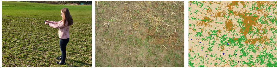
Figure 1.3: Left: Person capturing an image of the soil surface for soil cover estimation; Middle: image of the soil surface; Right: classification of the soil cover components in the image by a CNN
