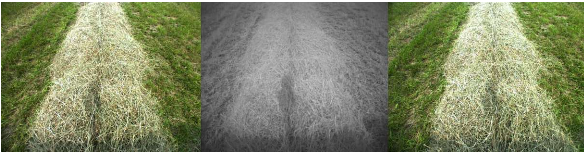
Figure 5.14: Captured images of a swath. Left RGB image, NIR image (850 nm) and right RGB image.
