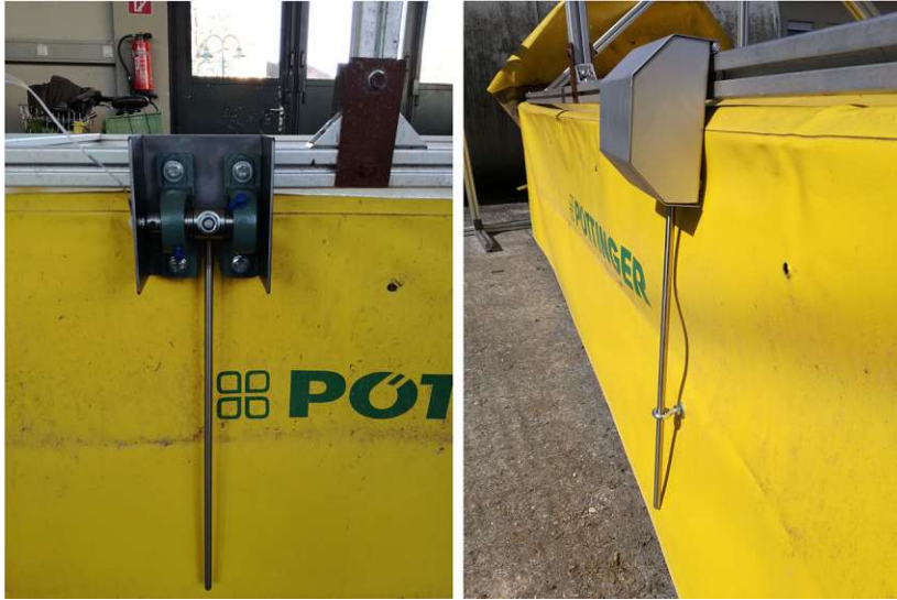
Figure 5.4: Pendulum-meter on the mower for measuring the deflection angle of the mower cloth.
