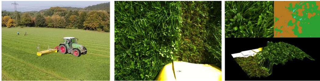
Figure 1.5: Left: Tractor and mower with cameras and sensors mounted; Middle: Camera view on the cut edge; Right: top: classification of legumes and grasses in the image, bottom: 3D stereo reconstruction of the scene for plant height measurement.
