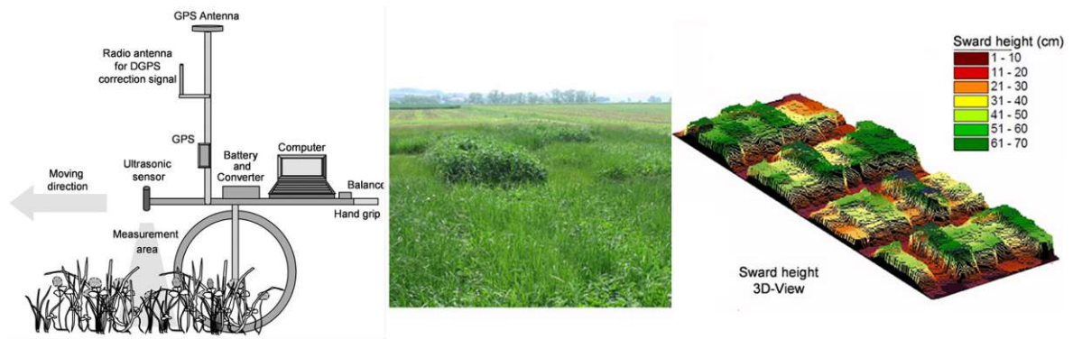
Figure 2.3: Images of the method proposed in [94]. Left: on-the-go application as a combined real time measurement of ultrasonic sward height and high precision GPS in movement; Middle: experimental layout; Right: point cloud of the sward height measurements with an ultrasonic sensor
