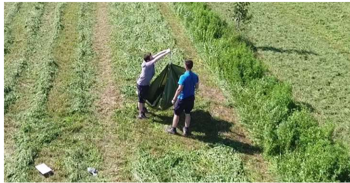
Figure 5.17: Manual weighing at random sample points during mowing and raking with the suspension scale and a tarpaulin.
