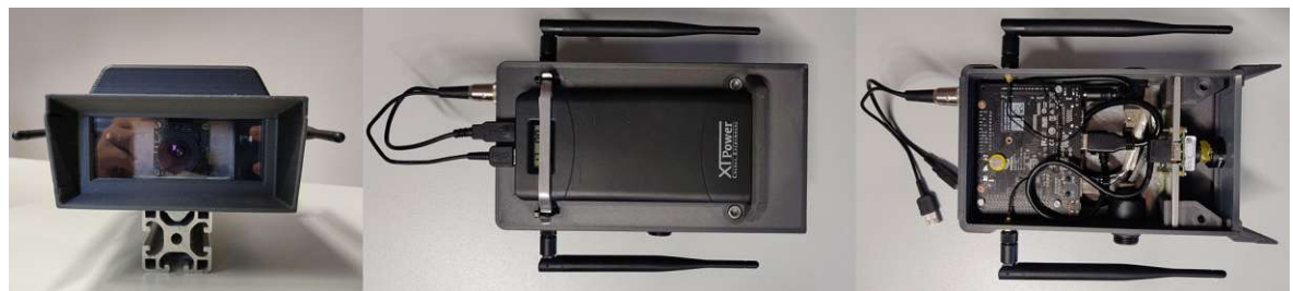
Figure 3.2: Hardware for capturing RGB images on a mobile machine. The system includes a DS RGB UI-3251LE-C-HQ camera and a NVIDIA Jetson Nano for inference of CNN models.
