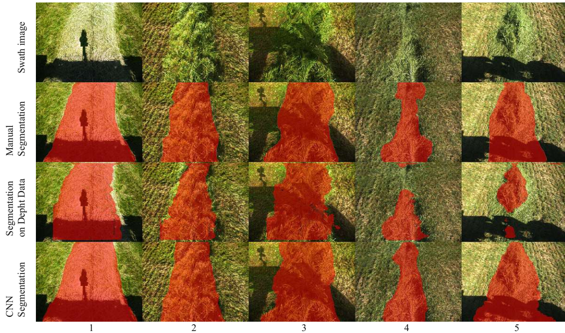
Figure 5.31: The swath segmentation results: the sample images followed by the manual labels, the segmentation results based on the depth data and the segmentation results based on the CNN
