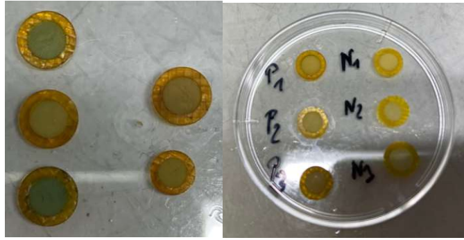
Figure 30: scaffolds after dissolving the heparin Toluidine Blue complex (left side first performed experiment, right side second performed experiment)
