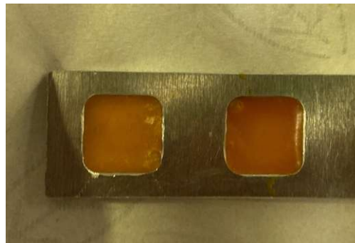
Figure 6: sample holder with 2 cutouts filled with the UPCL-6 resin
