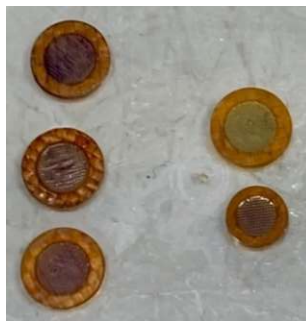
Figure 29: Toluidine Blue Quantification after the washing step to remove unbounded heparin, left-side heparin functionalized scaffolds, right-side control scaffolds without heparin
