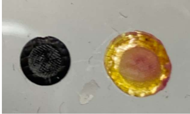
Figure 24: Ninhydrin assay: On the left-side aminolyzed scaffold, on the right-side non-aminolyzed control scaffold
