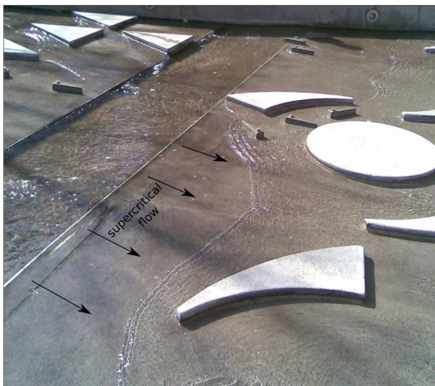
Figure 5.2: Observation of an undular hydraulic jump with convex front. Photograph taken by H. Steinrück in Karlsruhe, Germany on 24 March 2010.
