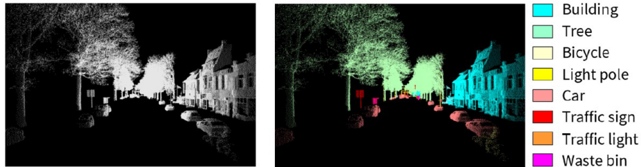
Figure 5.2: An example of raw point cloud collected by a mobile LiDAR sensor (left), and the classified point cloud (right).
