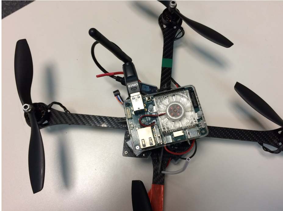
Figure 2-6 Odroid mounted on Hummingbird
