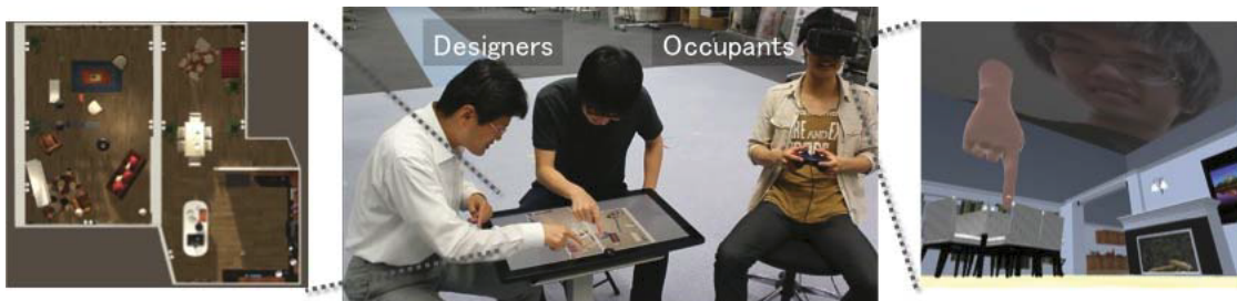
Figure 2.14: Virtual Dollhouse VR system by Ibayashi et al.: Top-down view for designers (left); All three collaborators using their devices (middle); VR view of occupant (right). Source: [ISS + 15]
