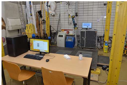
(a) Setup for test jumps: remote interaction console (front), simulation PC (back).
