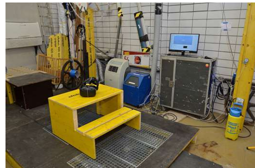
(b) Jumping area of the Jump Cube with stepping-pedestal and VR headset.
