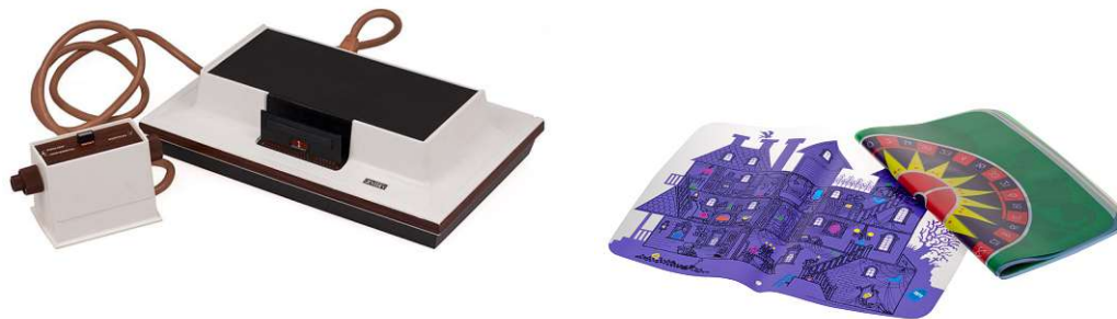
(a) Magnavox Odyssey video game console (one controller attached). Source: [Lan18] (b) Screen overlays that shipped with the Magnavox Odyssey . Source: [wik21c]
