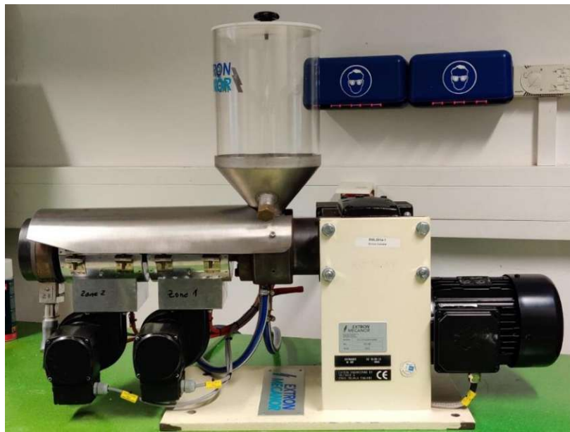
Figure 23: Extron EX-18-25-1.5 Lab Extruder for the reactive extrusion
