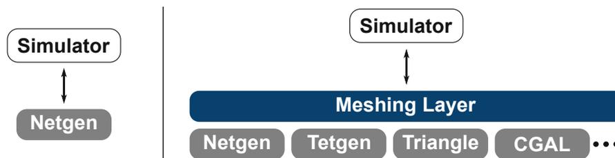
Figure 4.4: Interfacing a simulator with a single meshing backend limits flexibility with respect to mesh generation tasks (**left**). Instead, when a meshing layer is introduced, access to an expandable set of meshing backends is provided to the simulator via a unified interface (**right**).
