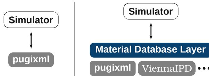
Figure 4.6: Interfacing a simulator with a single material database backend limits flexibility with respect to utilized material languages and access methods (**left**). Instead, when a material database layer is introduced, access to an expandable set of material database backends is provided to the simulator via a unified interface (**right**).
