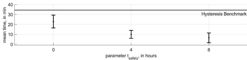
Figure 5.23: The time a HT is affected by an undercut of the SOC_{\min} is evaluated. The mean time per affected HT and the confidence interval of the execution with the EDCS and each parameter set is shown. The results are compared to the hysteresis benchmark. W = 36 simulation executions for each parameter set.
