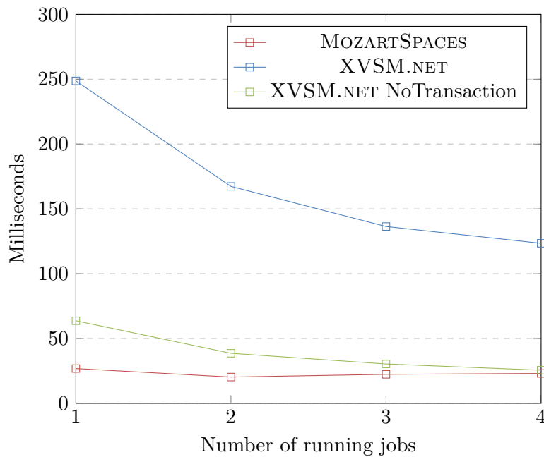
Figure 7.7: Performance of concurrent Read operations on a Label coordinator.
