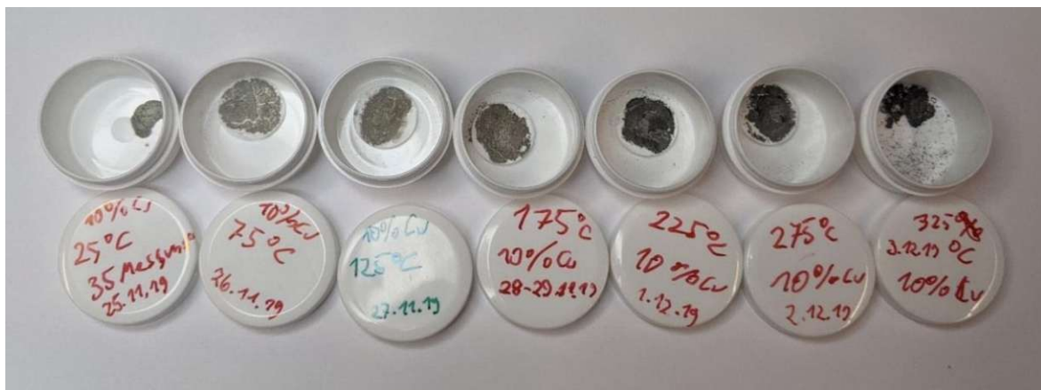
Figure 14: Corroded Samples of the Temperature Variation series prepared using synthesized \text{Ag}_2\text{O} and commercial \text{CuO} . Corroded using pressurized air and brine. Temperatures start with 25 °C on the left and increase in 50 °C steps. Picture taken 19 months after the original experiment.
