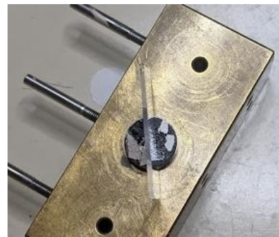
Figure 20: SEM sample holder loaded with both samples. Right: pure silver, left: silver + alumina
