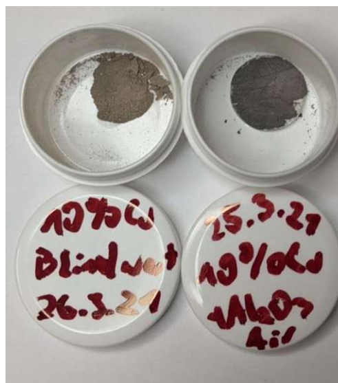
Figure 16: Corroded samples of the 10wCu+Al 2 O 3 series. One sample was measured under argon as a blind (left) and one corroded with air (right).
