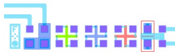
Figure 3.1: One flute (PQC main flute 1) with passivation openings for contacting shown in magenta.
