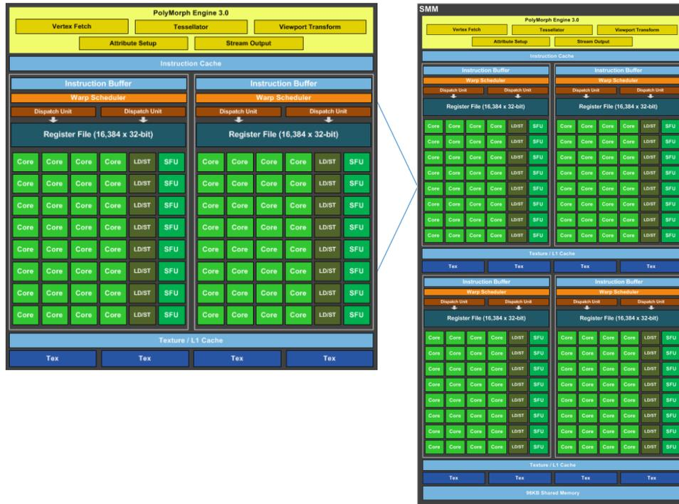
Figure 2.2: Maxwell Streaming Multiprocessor (SMM) (adapted from [NVI16]).
