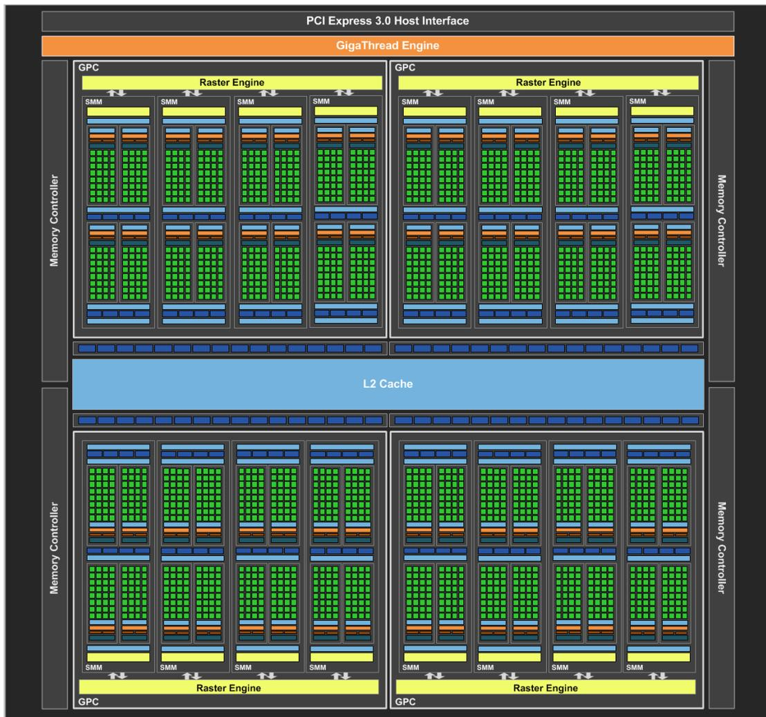
Figure 2.1: Block diagram of NVIDIA's Maxwell chip [NVI16].
