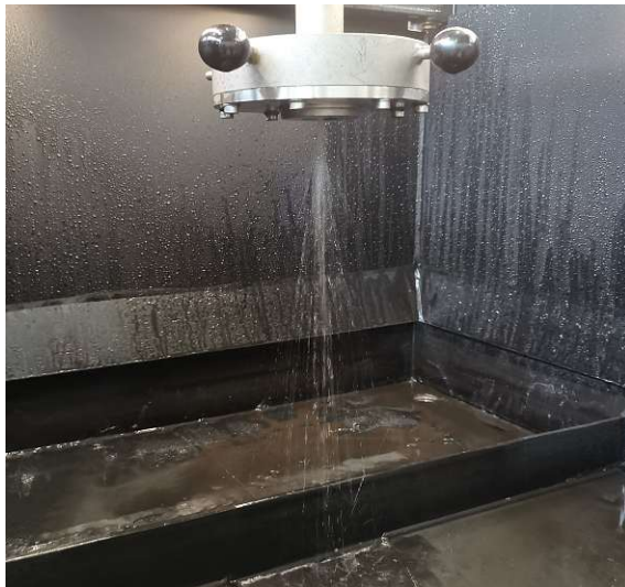
(a) Laminarer Strahlaustritt
