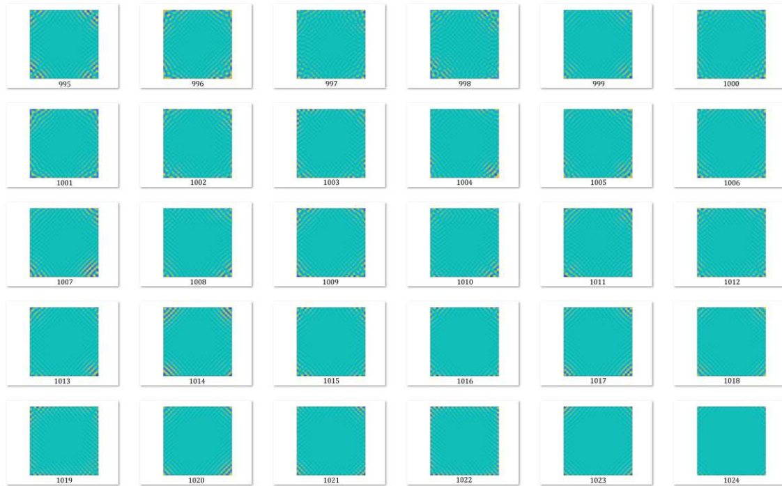
Figure 4.7.: The 30 most reflective eigenmodes of the reflection matrix of a 4 \times 75 mm 4f-cavity-CPA at critical attenuation, ordered by increasing reflectivity. Parameters: r_0^2 = 0.8 , \lambda_0 = 800 nm. Observation plane 2.5 \text{ mm} \times 2.5 \text{ mm} . Maximum modes: n_x = n_y = 16 . Lenses: aspherical . Propagation simulation: Rayleigh-Sommerfeld .
