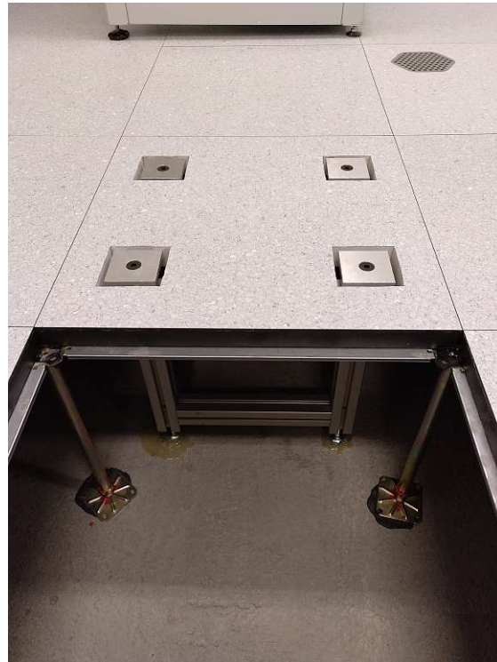
Figure 3.2: Aluminium pedestal to decouple the ORS from vibrations on the laboratory's floor.
