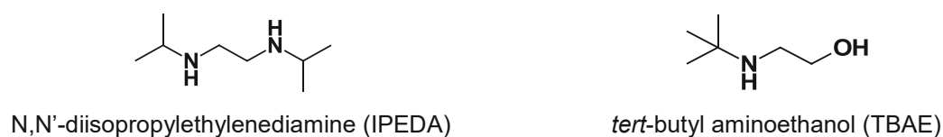
Figure 50: Structures of the second chain extenders used to introduce HUBs in the TPUU
