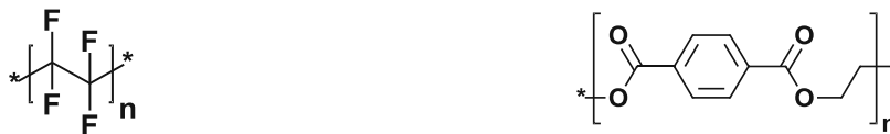
Figure 6: Repeating units of ePTFE (left) and PET (right) used as non-degradable scaffold materials
