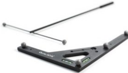
Figure 13: Example of calibration wand and L-frame from Qualysis [33]
