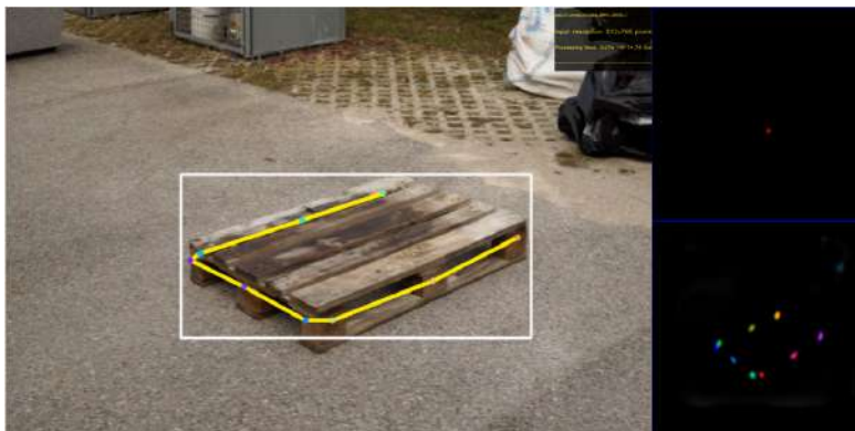
Figure 5.5: The left image shows a real-world input image, with the estimated bounding boxes and corresponding palette key points. The left upper heatmap visualizes the palette center estimate. The left lower heatmap shows the palette key point estimates.
