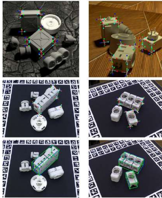
Figure 2.10: Visualization the 2D corner detection and corresponding 3D bounding box [PIL19]
