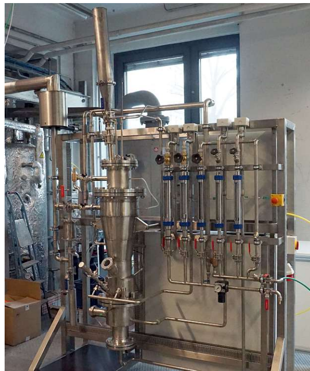
Figure 29: ICFB reactor in TU Wien research laboratory.
