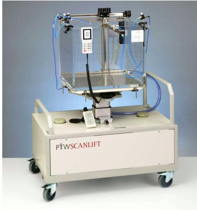
Figure 3.3: MP3-M water phantom system of PTW [PTW12]
