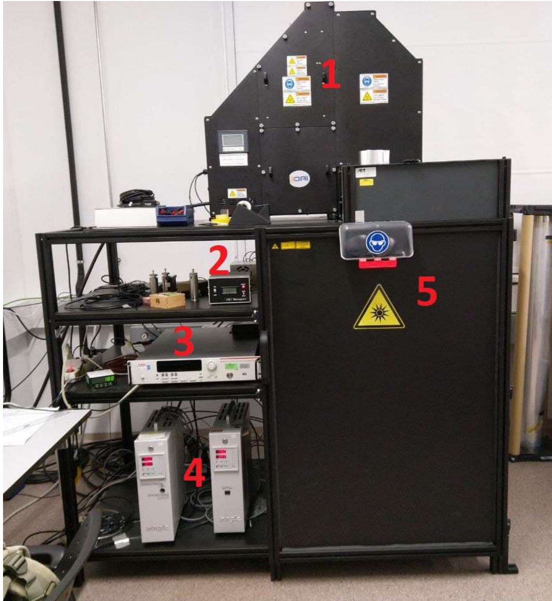
Figure 3.2: Setup of the small sun simulator, consisting of: [1] AAA class steady state solar simulator Xenon lamp, [2] temperature sensors, [3] high power series sourcemeter, [4] water cooling for lamp and sample and [5] the darkened chamber for measurements.
