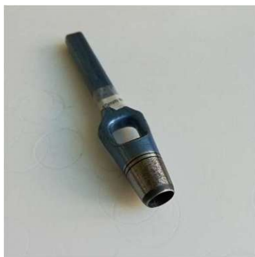
Figure 2.14 Metal punch used for the partition of the filter material for the 'ws'-ion and carbon content analysis
