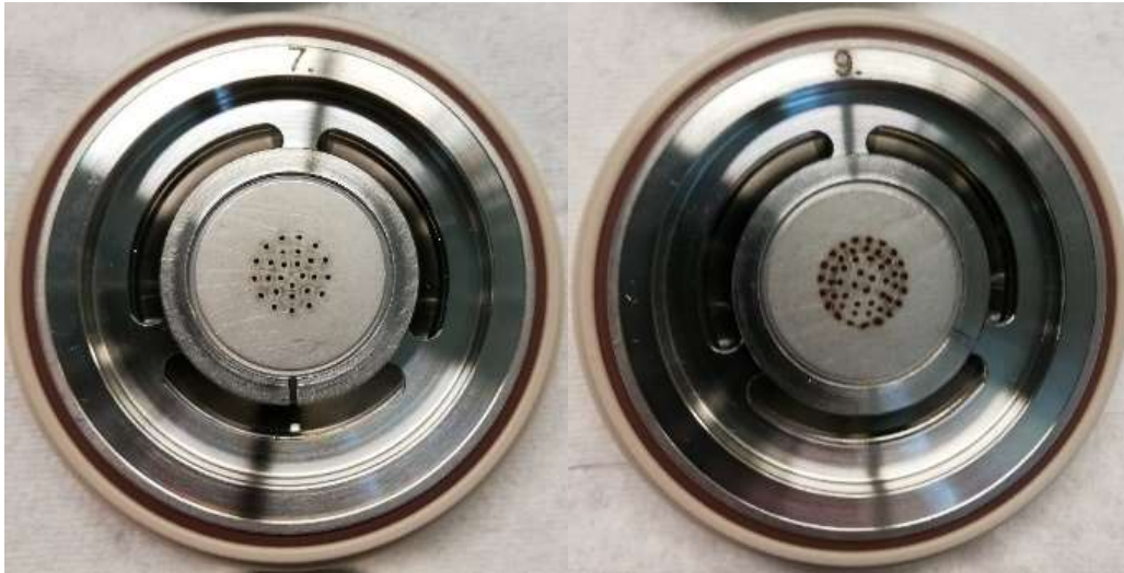
Figure 2.12 Impactor stage 7 with particles of an aerodynamic diameter between 155 and 256 nm (left) and stage 9 with particles with an aerodynamic diameter between 382 and 603 nm (right) of the electrical low-pressure impactor after the measurement at tunnel Praterstern U2
