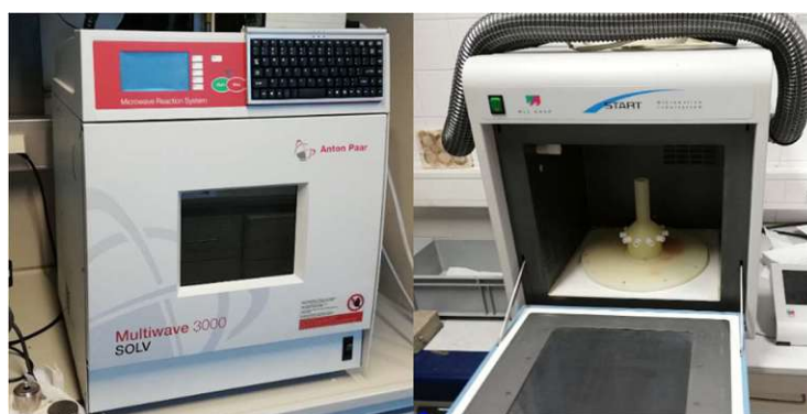
Figure 2.17 Microwave A (left) and microwave B (right) used for the filter digestions
