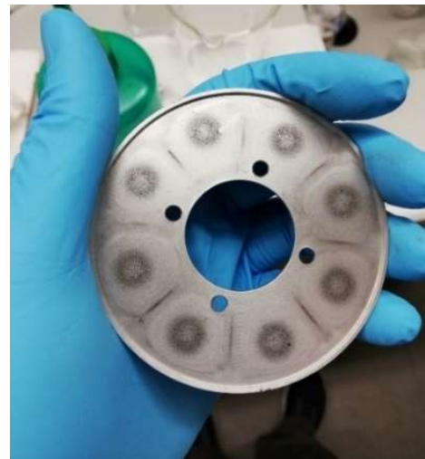
Figure 2.2 Impactor plate of the Low volume sampler with the collected dust (aerodynamic diameter >10µm)
