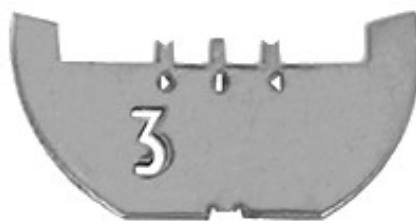
Figure 2.6: A typically used Mo FIB-lamella sample holder.
